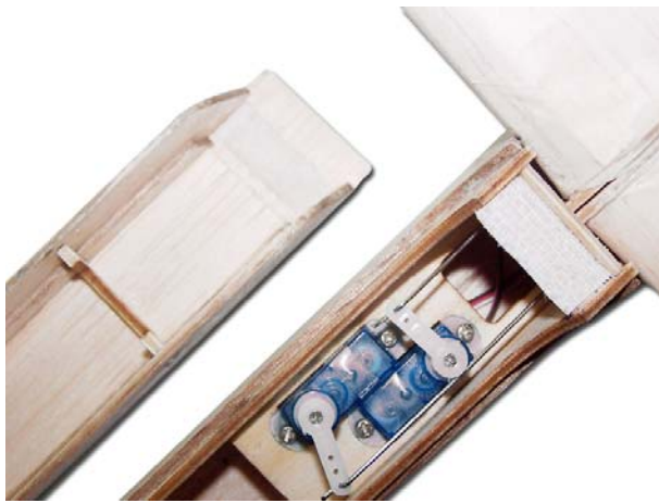
Turn on the power and four servos should work properly.
